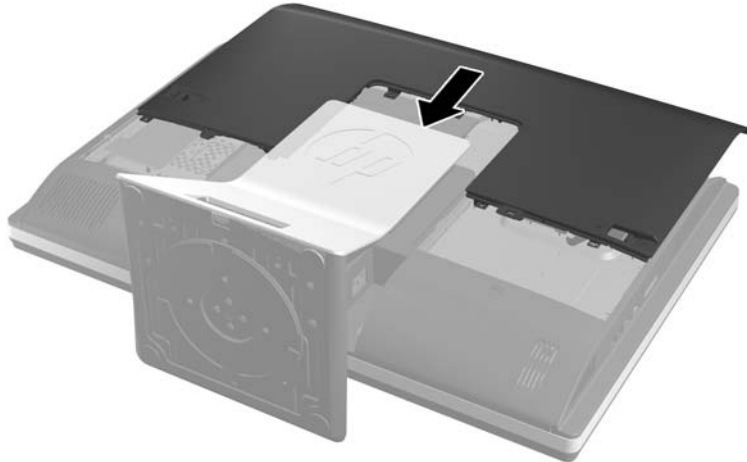
Figure 6-12 Replacing the access panel
